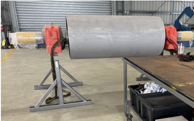
Bare pulley shell in the workshop.
