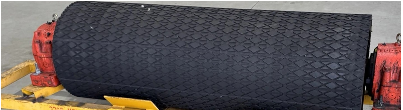
Diamond-pattern lagging on a pulley in the Superior workshop.
