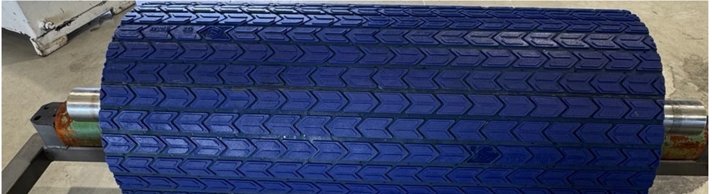
Blue polyurethane lagging on a pulley in the Superior workshop.
