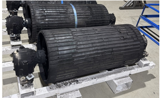
Pulley assemblies in the workshop.
