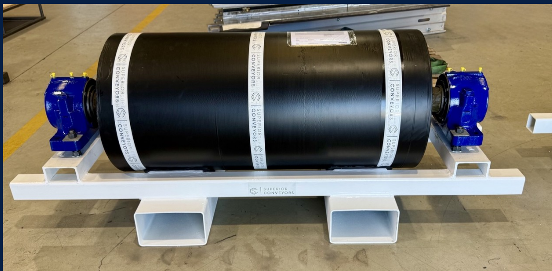
Completed pulley assembly on a transport cradle in the Mackay workshop.
