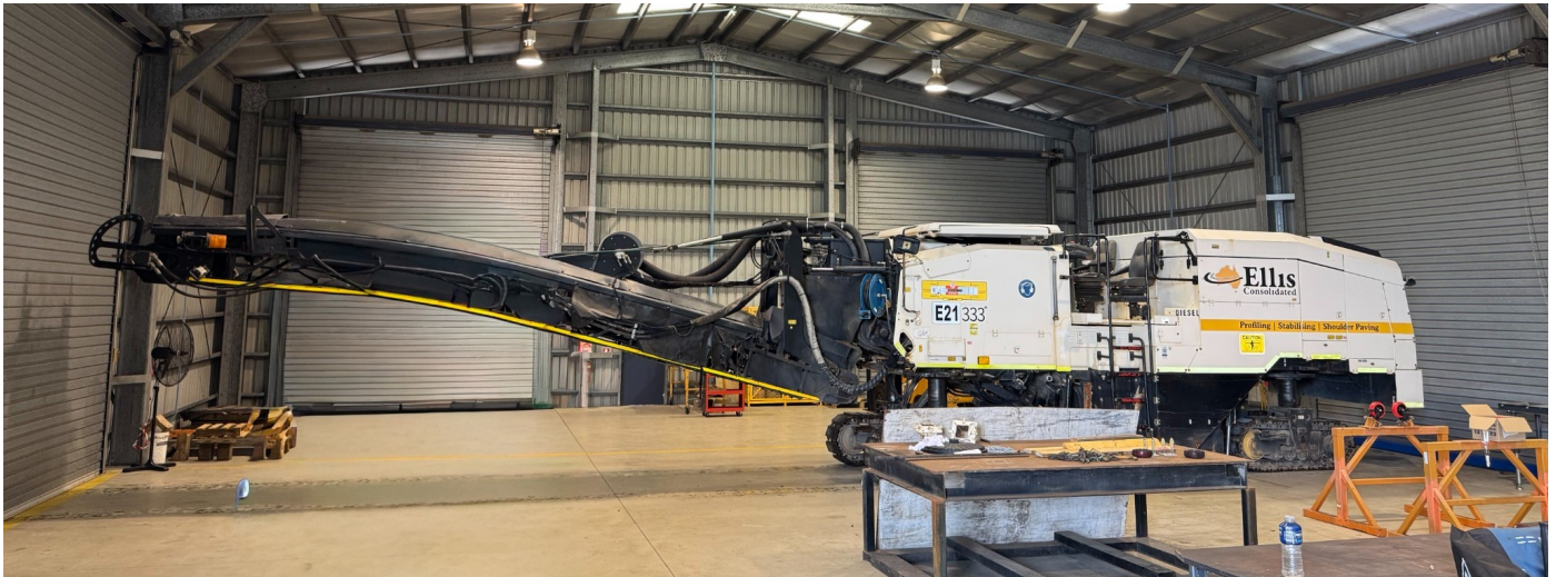
Road-profiling machine and discharge conveyor in the workshop.
