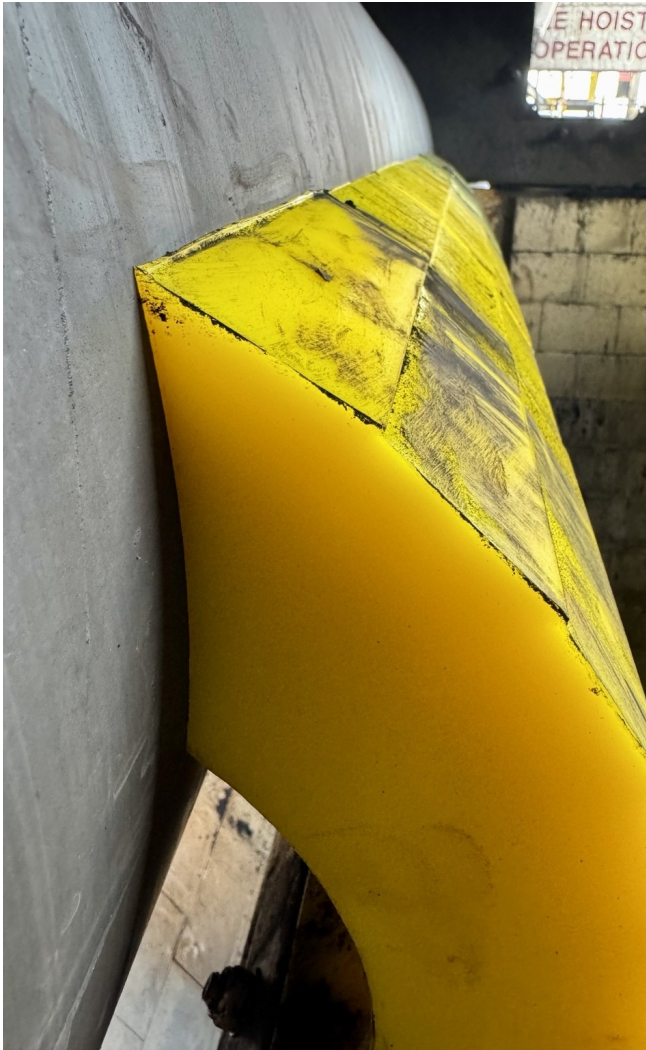
Super XHD polyurethane blade working against the pulley-supported belt.
