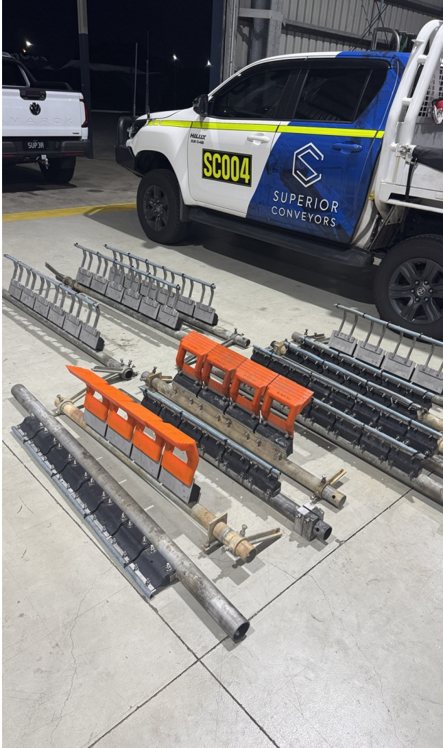
Polyurethane suspension-arm assemblies prepared alongside tungsten-tip cleaners.
