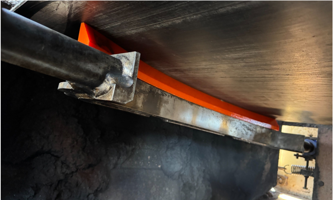
Curved secondary cleaner with an orange polyurethane blade installed against the belt.
