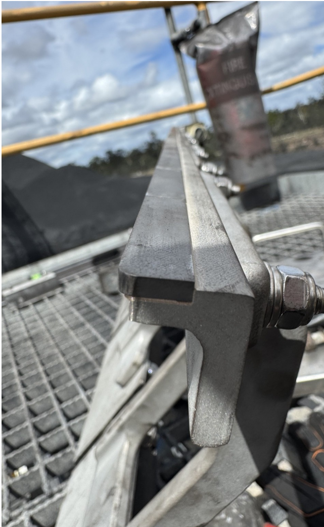
Tungsten tip secured to its suspension arm.
