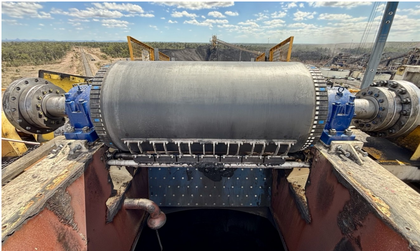
Primary Head Cleaner installation in the head chute; removed material falls back into the process.
