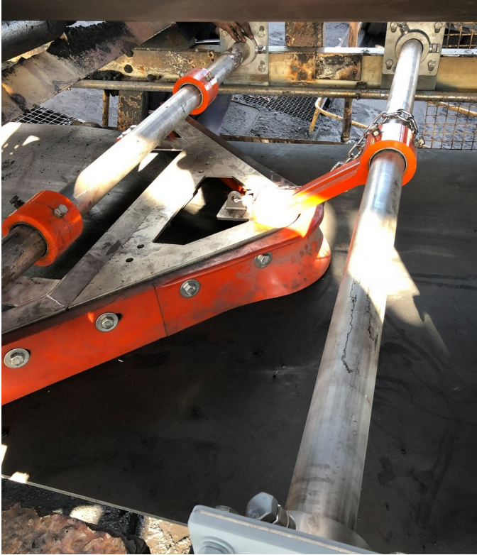
V-plough installations showing blades, support poles and restraint components.
