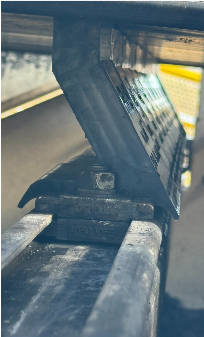
Inline secondary cleaner showing the wear segment secured to the slide frame.
